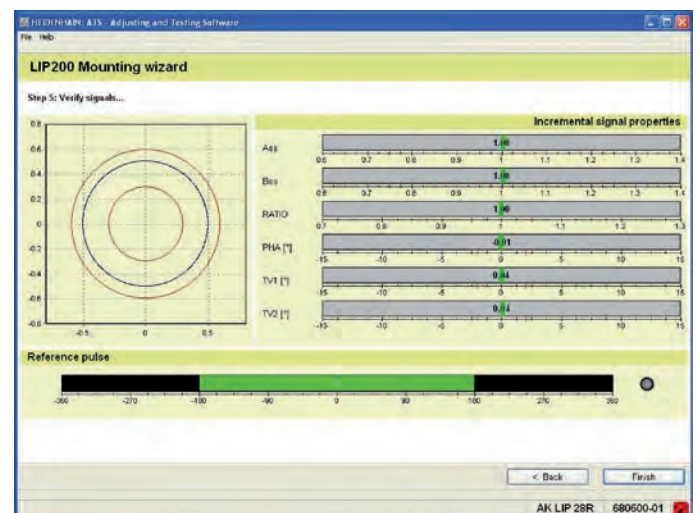
Commissioning with the PWM 21 and ATS software
