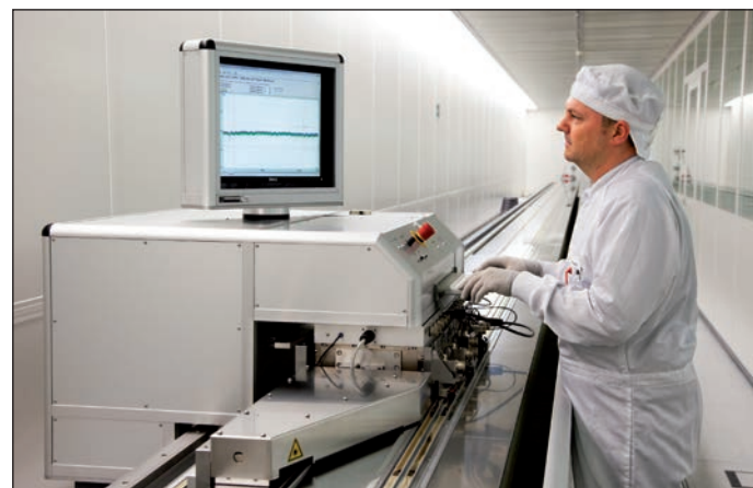
30 m long measuring machine for scale tapes
