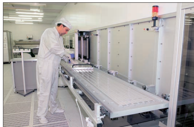
Vacuum machine for application of chromium layers
