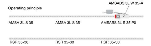
The operating principle is built on the proven products AMS 3L and AMSABS 3B. A measuring carriage AMSABS 3L W with absolute measuring reading head runs over rail butt-joints without loosing the signal. The single rail segments have a standardized length L3 and are prepared for joints on both sides. This allows to arrange the rails one by one in any length and random sequence.
