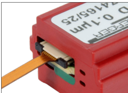
Correctly inserted sensor print
