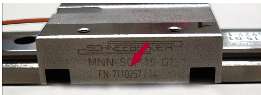
The carriage number is printed on the label of the interface module
